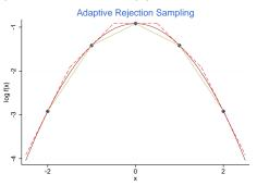
The method samples from the outer envelope, accepts values under the inner envelope, and otherwise evaluates f(x) to decide and then f'(x) to tighten the envelopes.
